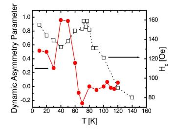
FIG. 7. (Color online). Temperature dependence of the dynamic loop asymmetry parameter, as defined in the text (left axis, solid points). The coercivity extracted from conventional magnetometry measurements is shown for comparison (right axis, open points).
