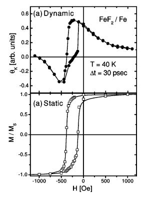
FIG. 5. (a) Dynamic hysteresis loop for FeF<sub>2</sub>/Fe at T=40 K. These data were taken at a fixed delay between field and probe pulses of 30 ps. (b) Static hysteresis loop (from SQUID magnetometry) at T=40 K.
