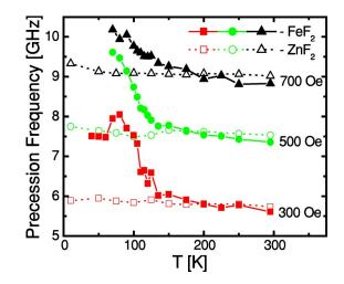
FIG. 4. (Color online). Temperature dependence of the characteristic precession frequency for  $FeF_2/Fe$  (solid points) and  $ZnF_2/Fe$  (open points) for applied dc magnetic fields of 300, 500, and 700 Oe. These data are extracted from curves of the type shown in Fig. 3 after Fourier transformation of the raw time dependence data.
