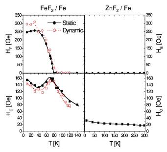
FIG. 2. (Color online). Temperature dependence of the exchange bias ( $H_E$ ) (top panel) and the coercivity ( $H_C$ ) (bottom panel) for FeF<sub>2</sub>/Fe (AF/FM) (left panel) and ZnF<sub>2</sub>/Fe (nonmagnetic/FM) bilayers (right panel). Solid points are from conventional SQUID magnetometry while the open points are from dynamic hysteresis loops as discussed in the text.
