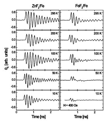
FIG. 3. Time dependence of the Kerr rotation,  $\theta_K$ , for ZnF<sub>2</sub>/Fe (left panel) and FeF<sub>2</sub>/Fe (right panel). The data were taken from 295 K (top) to 10 K (bottom). The applied dc magnetic field is 400 Oe.
