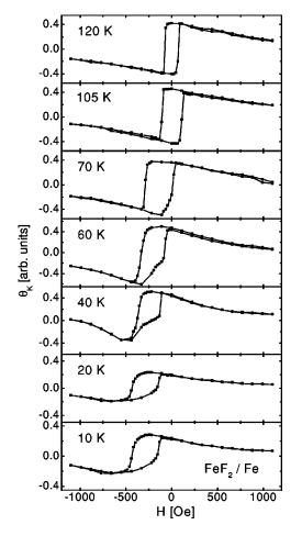
FIG. 6. Temperature dependence of the dynamic hysteresis loops for  $FeF_2/Fe$ . These data were taken in a similar manner to those shown in Fig. 5.
